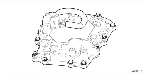
13) Disconnect the harness connector from the control valve body.
