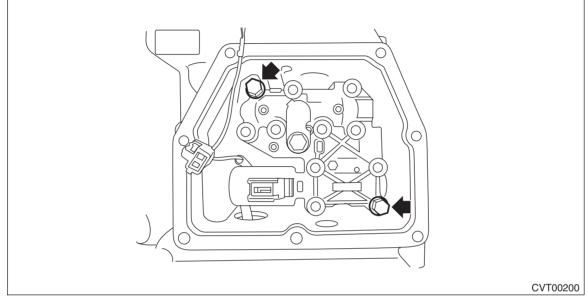
(2) Install the bolt and the ground terminal.
