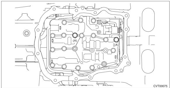
5) Install the O-ring to the transmission harness.
