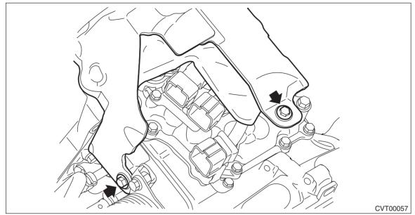
8) Remove the transmission harness stay, drive motor harness stay and transmission ground terminal.
