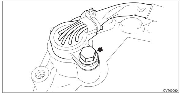
15) Remove the O-ring from the transmission harness.
