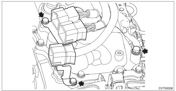
9) Remove the transmission harness connector from the harness stay.
