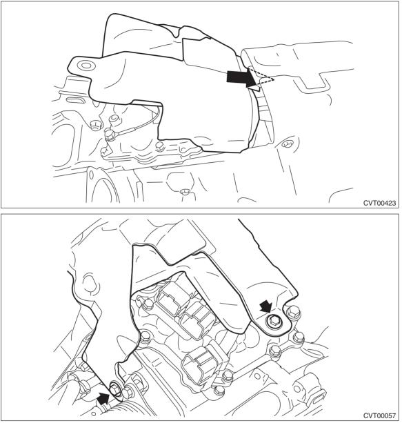
14) Install the pitching stopper bracket and transmission radio ground cord.
