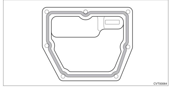
7) Install the oil pan by equally tightening the bolts.
