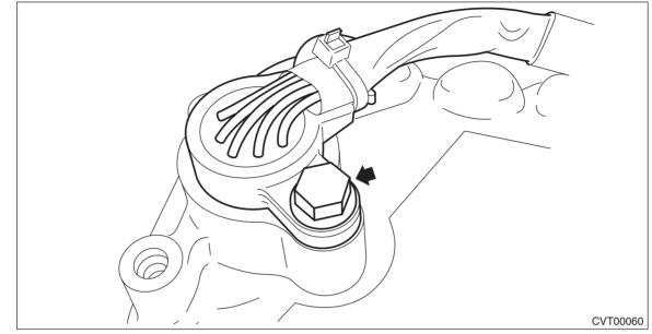
7) Install the gasket to the transmission.
